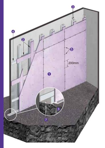
FRL resistance -/240/-BS EN 1364: Part 1: 1999 Standard BS EN 1363: Part 1: 1999 Fire IT 14-1919 Approval **FORTE** Maximum 6000mm height Construction Partition Unlimited length Partition Nominal 68mm thickness
