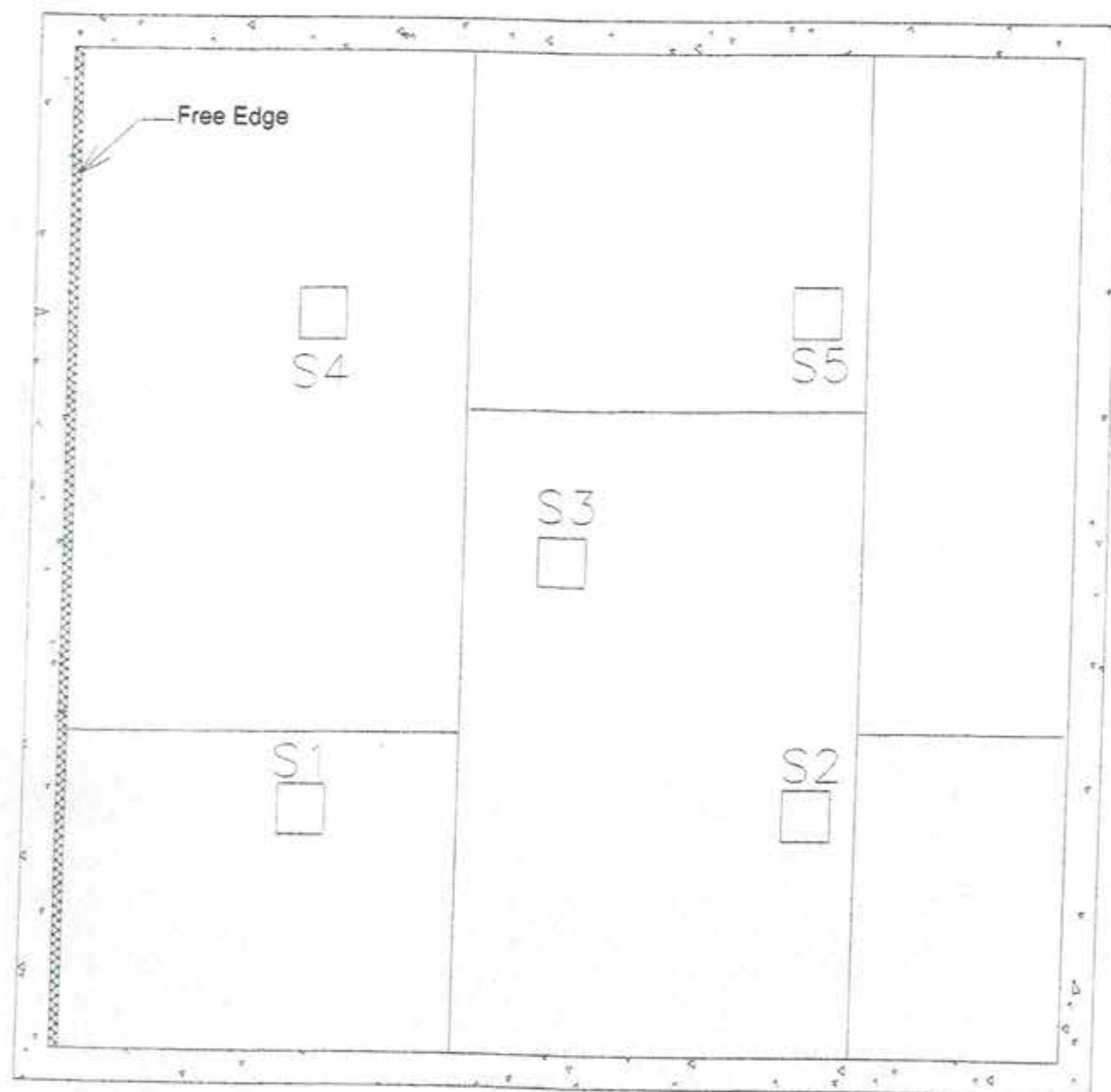
Figure 2 – Locations and reference number of thermocouples to monitor the temperature of unexposed surface of the specimen.
